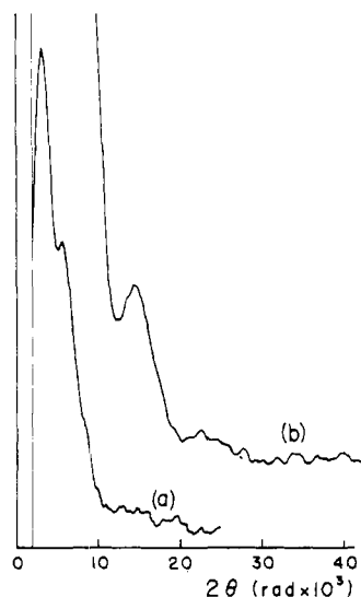
Figure 14. Small-angle X-ray scattering curve measured on a Kraton-G film cast from heptane, stretched at \epsilon = 1 . Intensity measured in the same direction as the extension direction. Exposure time: (a) 5 h, (b) 48 h.
